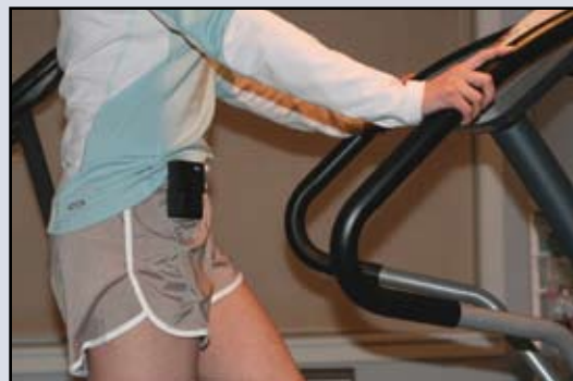
Figure 3. UbiFit employs the Mobile Sensing Platform as a fitness device to automatically infer physical activities.
